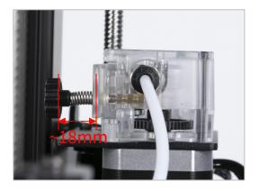
Note: The better distance for extruding filament is about 18 mm.You may adjust the distance of the screw for the different filament.
