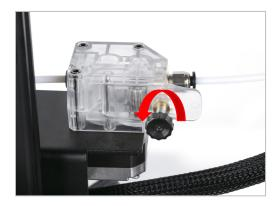
If the melted filament is too thin, please reduce the extrusion force by rotating counterclockwise.
